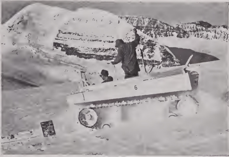
FIGURE 30. "Inherent increase of climb" of about 4 degrees is evident in downhill runs by pilot model of T-15 Weasel.
